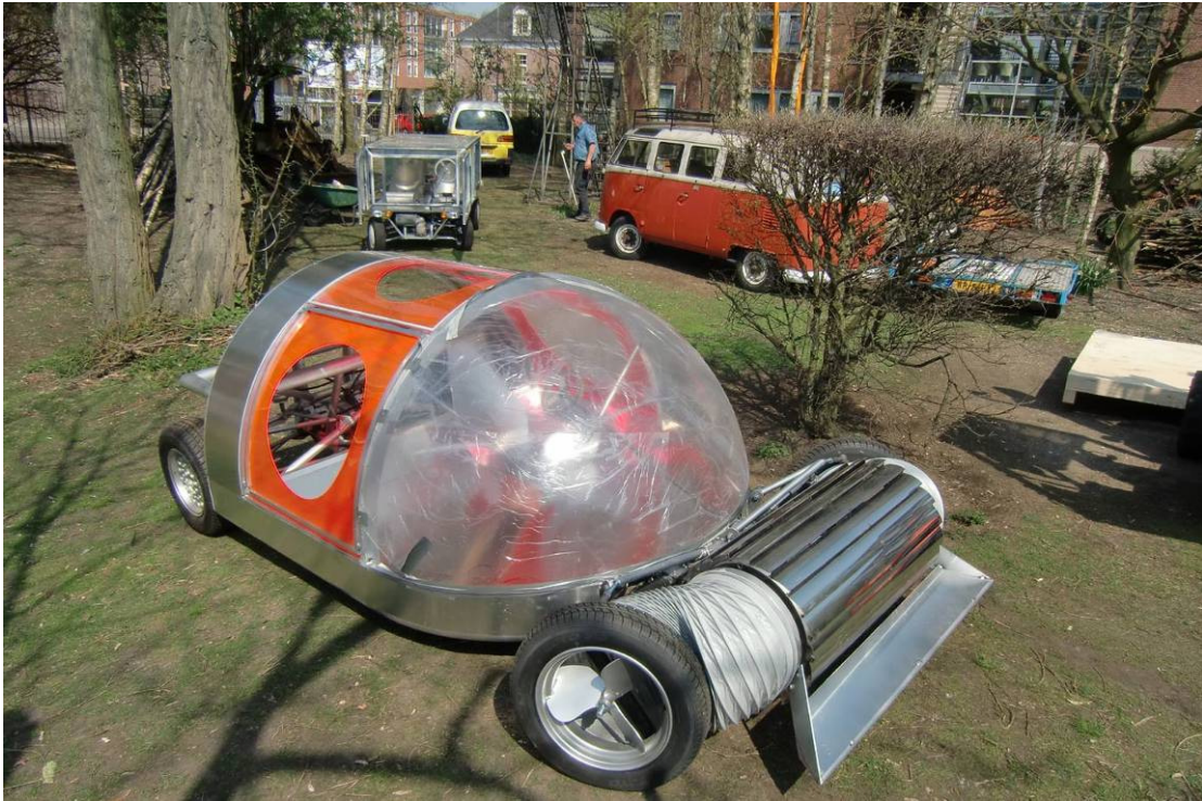
Wind Turbine Car; spoiler, wind turbine, suction by the front wheels
